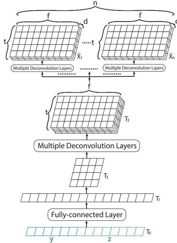
Fig. 3. The neural network design of SenseGAN generator.
